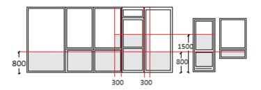
Always choose personal safety glass if part of the unit is placed less than 1.50 metres above the floor in doors and door side-lights and access points. The same applies to other risk areas where the unit is placed less than 0.8 metres above a particular surface. Guidelines for safety glass are described in BS 6206:1981 and BS 6262-4:1994
